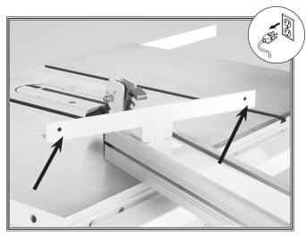
Figure 13. Fence adjustment setscrews.
